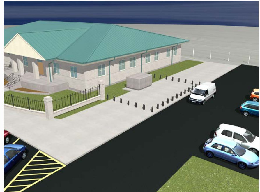
Example of standoff distance enforced with the use of bollards
